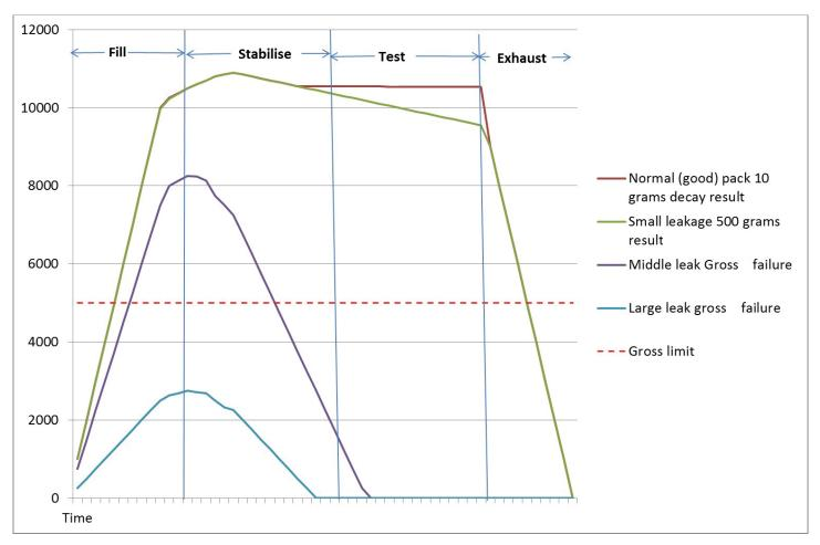
By monitoring the force, the result by force decay can also determine approximate hole size which could be considered under the salvage option (yellow lamp, if fitted). Results can either be logged to USB, Ethernet or to a printer, using the pre-written format or can be edited to meet individual needs.
