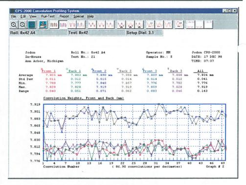
The CPS chart shown above displays individual heights and a statistical summary of a 50-convolution sample. Front and back results are shown for each of 3 regions across the width. Regions 1 and 3 represent the height near the top and bottom of each convolution. Region 2 measurements are from the midpoint of each convolution. (Note that region 2 is approximately 80 microns larger than regions 1 and 3.)
